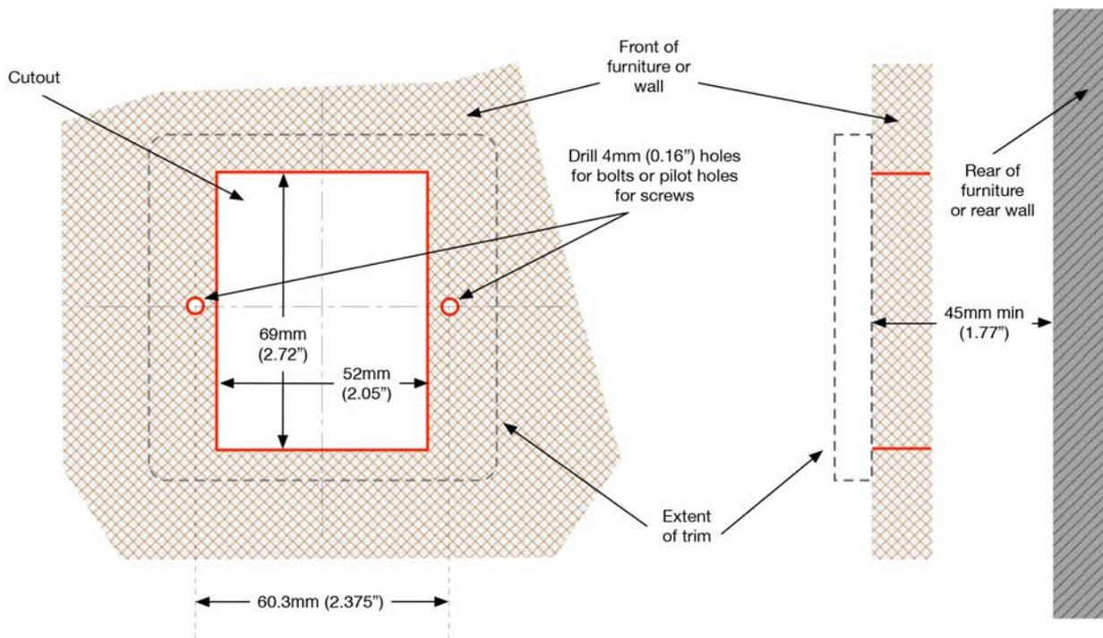
**Step 2.** Ensure HDMI and DC power are presented at the cutout and that you have sufficient slack to allow connection to the rear connectors on MediaHub UHD main unit. **Ensure the PSU is NOT plugged into the mains at this point.**
